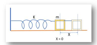
Let the system be displaced through a distance X. (<u>Note</u>: You are also free to use small letter 'x' for displacement for consistency through the chapter of SHM). Then a restoring force is developed such that the system has the tendency to come back to the mean position.
