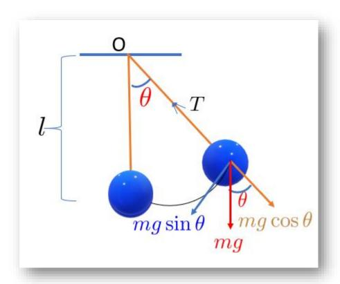
A simple pendulum consists of a metallic bob suspended with an extensible thread or rope at the point O. It is displaced through a small angle  $\Theta$ .
