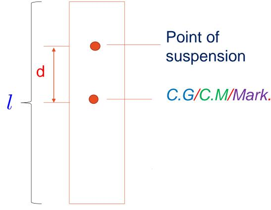
d is the distance between the point of suspension and the C.G.
